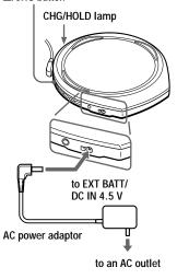
The CD player charges the batteries. The indicator sections of with in the display of the remote control light up in
